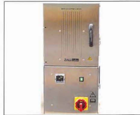
Figure 6. Zirkonzahn's specific sintering oven for Prettau zirconia.
