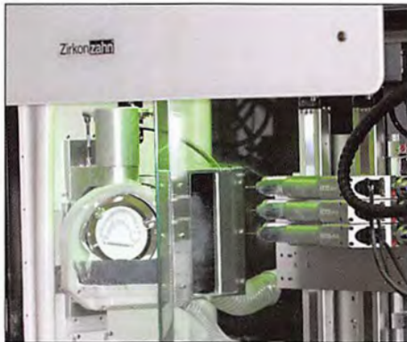
Figure 5. Zirkonzahn's specific 5-axis zirconia milling machine for Prettau zirconia.
